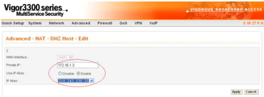
Figure 36-6. The second DMZ Host configuration
