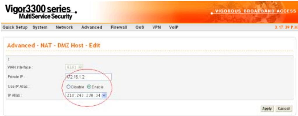
Figure 36-5. The first DMZ Host configuration
